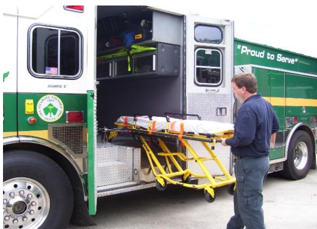
Photo of Combination pumper-ambulance in Sycamore Township, Hamilton County, Ohio. This has merit in some departments but is not recommended for Hubbard because of cross-contamination in two directions (fire debris to patients and patient pathogens to firefighters.)
